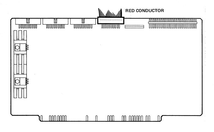
Figure 3-6: 20-Pin Cable Connection (P2 -P5)
