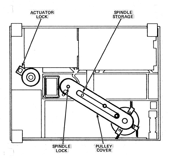
Figure 3-8: M26 Disk Drive (Spindle Lock and Actuator Lock)
