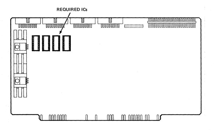
Figure 3-11: HDCA Controller Board (Location for Required ICs)
