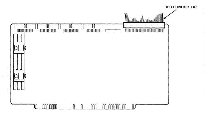
Figure 3-5: 50-Pin Cable Connection (P1)
