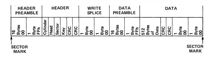
To maximize the transfer of sectors to the host computer system's memory, Morrow Designs software uses a physical sector skew when formatting the drive. This skew takes into account the time required to transfer a sector of data into memory using I/O instructions, and will allow the operating system to read more than one sector per disk revolution. The Morrow Designs skew table is illustrated in Table 5-3.
