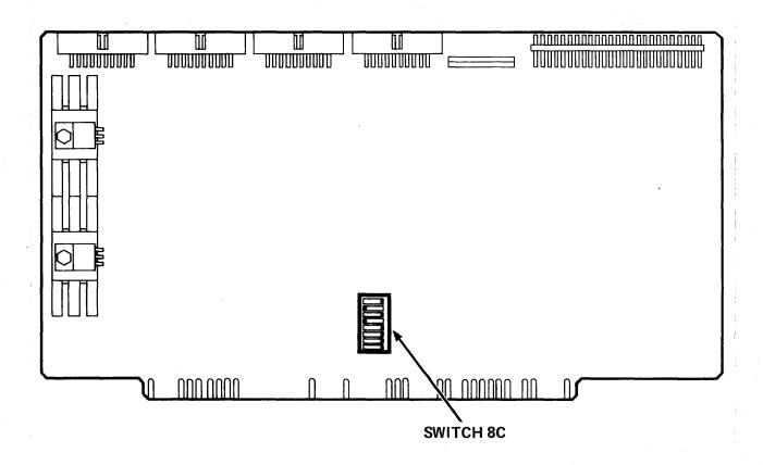
Figure 3-1: HDCA DIP Switch Location
