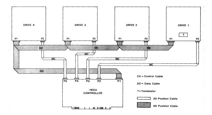
Figure 3-10: Multiple Drive Connection
