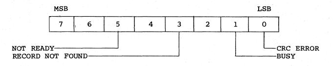
The "RECORD NOT FOUND" bit indicates that the external software has not selected the proper key to access the sector in question. If the "RECORD NOT FOUND" bit is set, the "CRC ERROR" bit should also be set. On rare occasions, error bits 0 and 3 will indicate that the header of the sector contains bad data or that a flaw exists in the magnetic media at this area of the sector.
