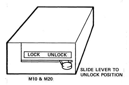
Figure 3-9: M10/M20 Disk Drive (Location of Head Lock) Locate the disk drive head lock, as illustrated in Figure 3-9.
