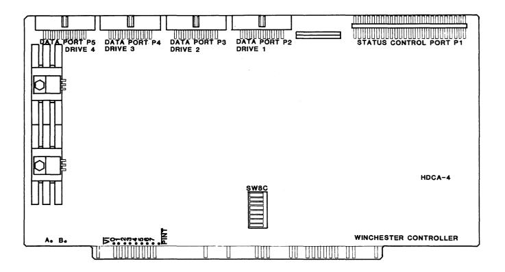
HDCA-4 Hard Disk Controller Component Layout
